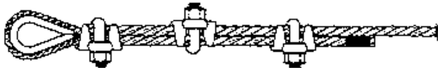
Wrong Way: Clips Staggered
