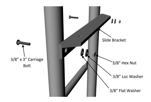
2. Attach the slide to the bracket by placing the slide in place on bracket. Then drilling with a 3/8" drill bit through the holes in the bracket into the slide. (Holes in the bracket should line up with mold for holes in the slide.) Then insert the BHS bolt through the slide holes and through the holes in the bracket. Then secure with the flat washer, loc washer, and hex nut. AS SHOWN ON RIGHT.
