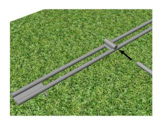
Start by placing seat upside down on ground. Slide the cross piece through the seat pivot, followed by the retaining rings. They should be almost touching teeter totter seat pivot. (one on each end) Then place the legs on each end. Once all pieces are equally spaced, insert and tighten all set screws. Turn the teeter totter over and mark the holes, dig, level out and mix concrete.
